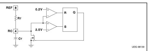
The UCC3813-0/-1/-2/-3/-4/-5 oscillator generates a sawtooth waveform on RC. The rise time is set by the time constant of RT and CT. The fall time is set by CT and an internal transistor on-resistance of approximately  $125\Omega$ . During the fall time, the output is off and the maximum duty cycle is reduced below 50% or 100% depending on the part number. Larger timing capacitors increase the discharge time and reduce the maximum duty cycle and frequency.
